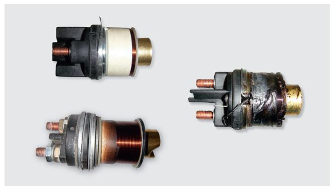
Figure 2: Indicator paper not discolored (top left), clearly discolored (bottom left), and a defective solenoid with charred indicator paper (right)
